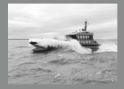
Vessels are designed to be self-righting. This capability has been successfully verified in real life tests.
